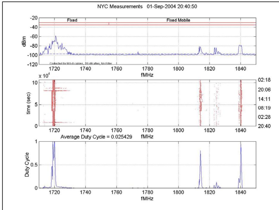
**Figure 51: September 1 to September 3, 1710 MHz – 1850 MHz**
