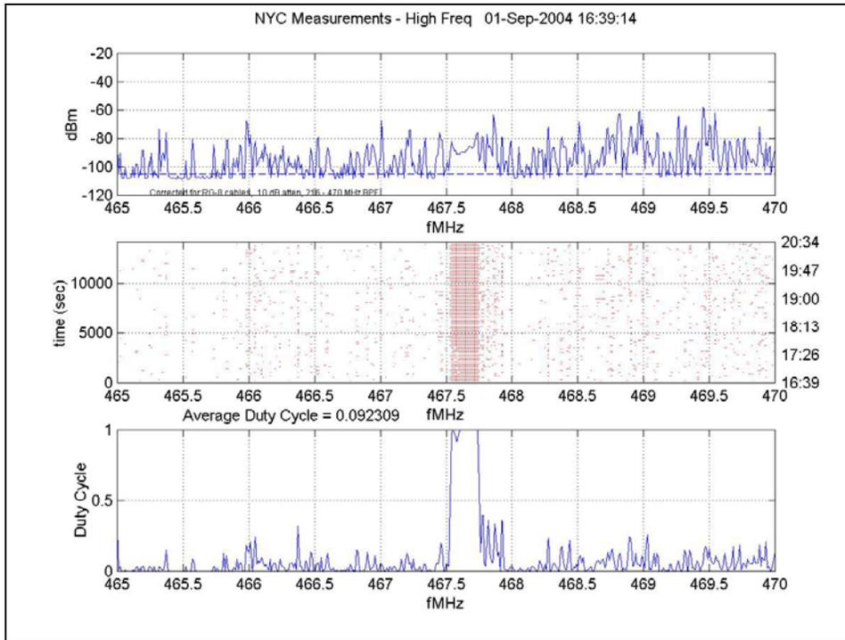
Figure 142: Small Frequency Resolution, 465 MHz – 470 MHz
