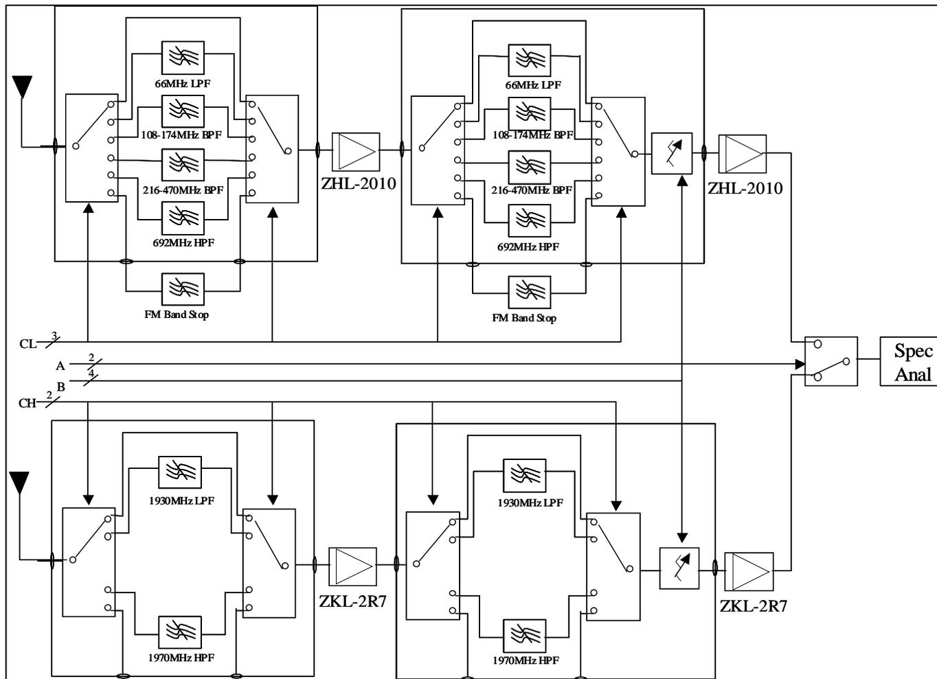
**Figure 4: Pre-Selector Block Diagram**
