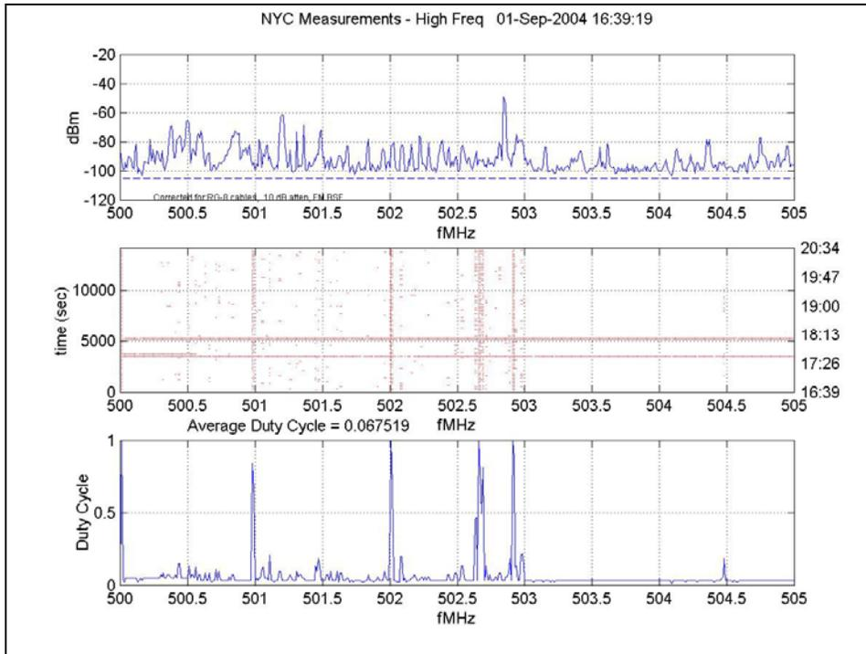
Figure 144 : Small Frequency Resolution, 500 MHz – 505 MHz
