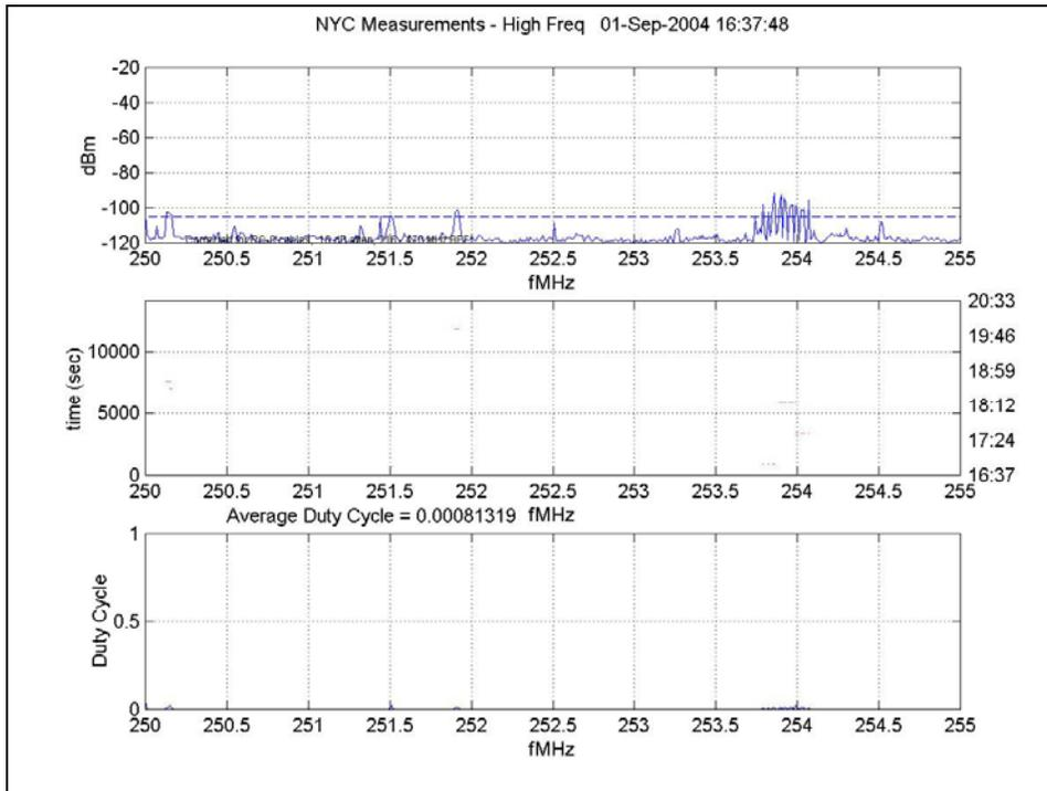
Figure 99: Small Frequency Resolution, 250 MHz – 255 MHz
