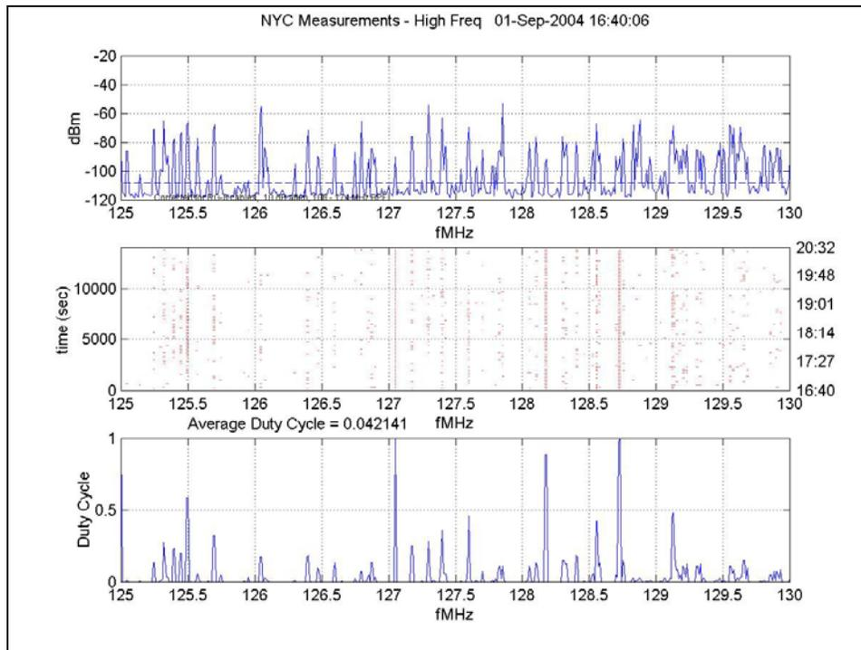
Figure 80: Small Frequency Resolution, 125 MHz – 130 MHz
