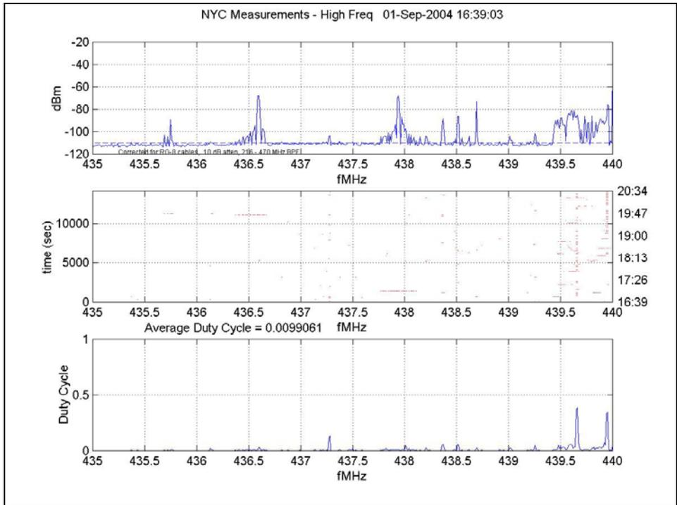
Figure 136: Small Frequency Resolution, 435 MHz – 440 MHz
