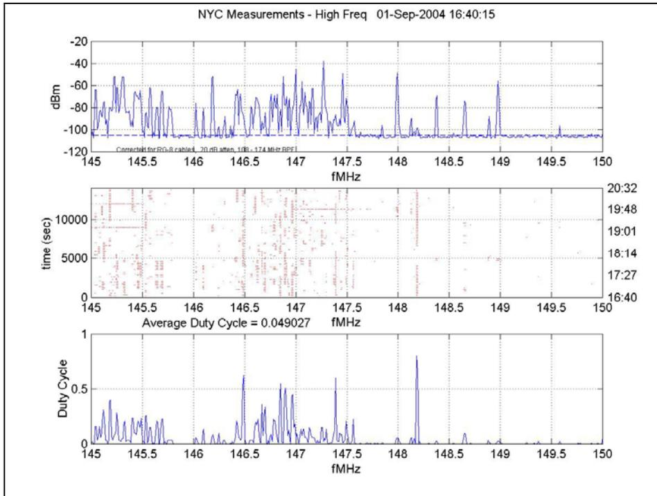
Figure 84: Small Frequency Resolution, 145 MHz – 150 MHz
