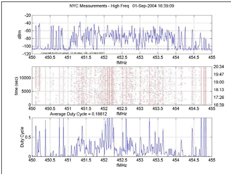
Figure 139: Small Frequency Resolution, 450 MHz – 455 MHz
