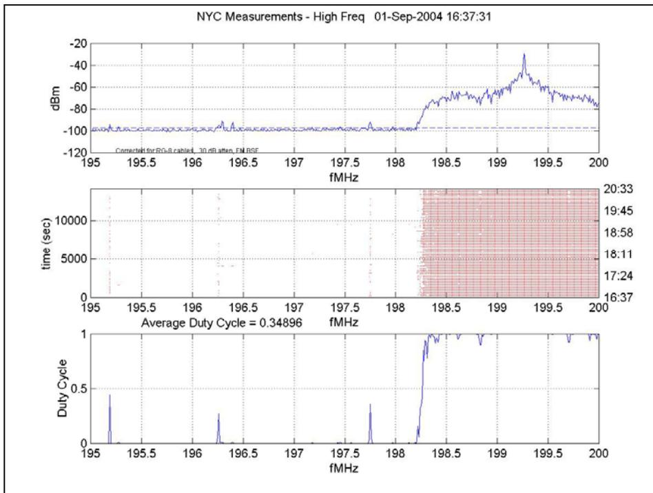
Figure 91: Small Frequency Resolution, 195 MHz – 200 MHz
