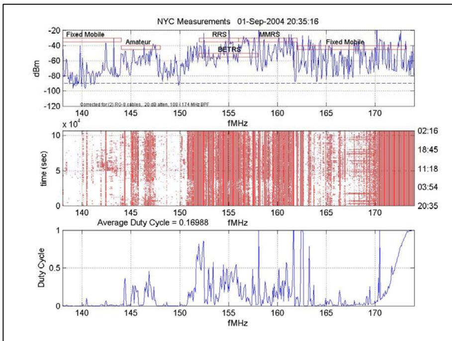
Figure 17: September 1 to September 3, 138 MHz – 174 MHz
