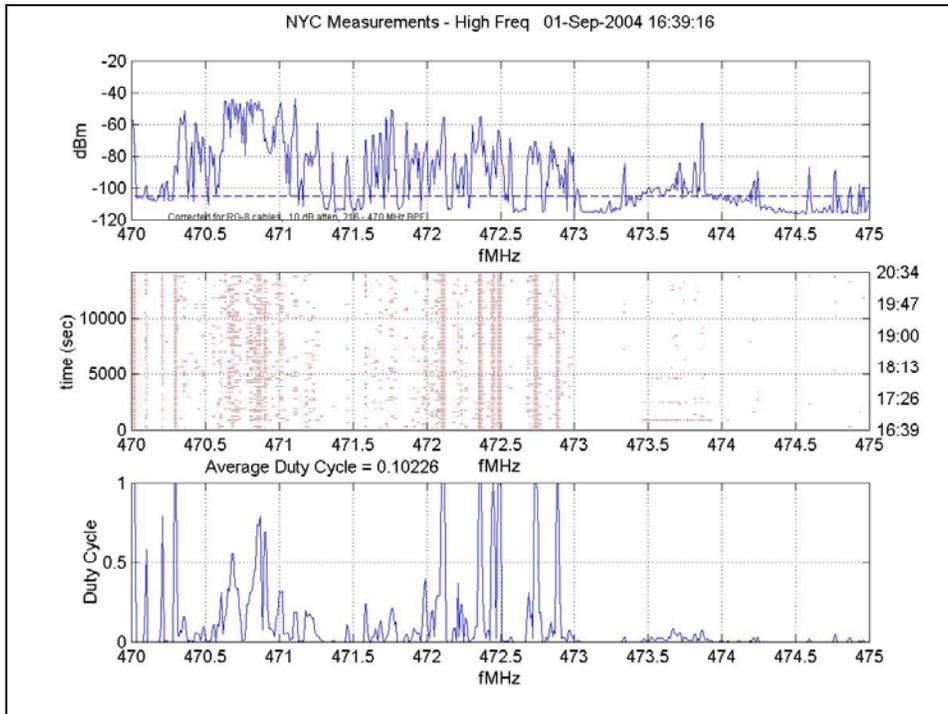
Figure 143: Small Frequency Resolution, 470 MHz – 475 MHz
