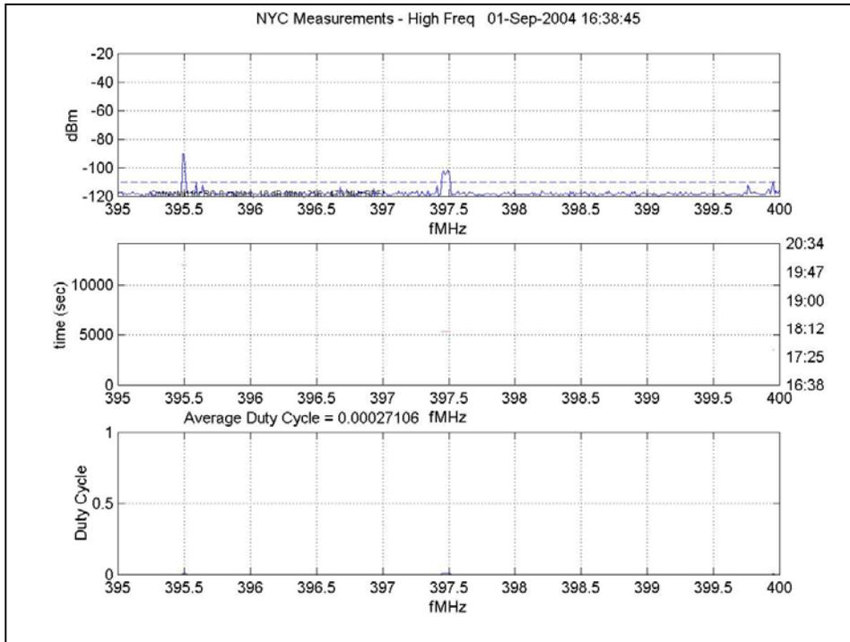
Figure 128: Small Frequency Resolution, 395 MHz – 400 MHz
