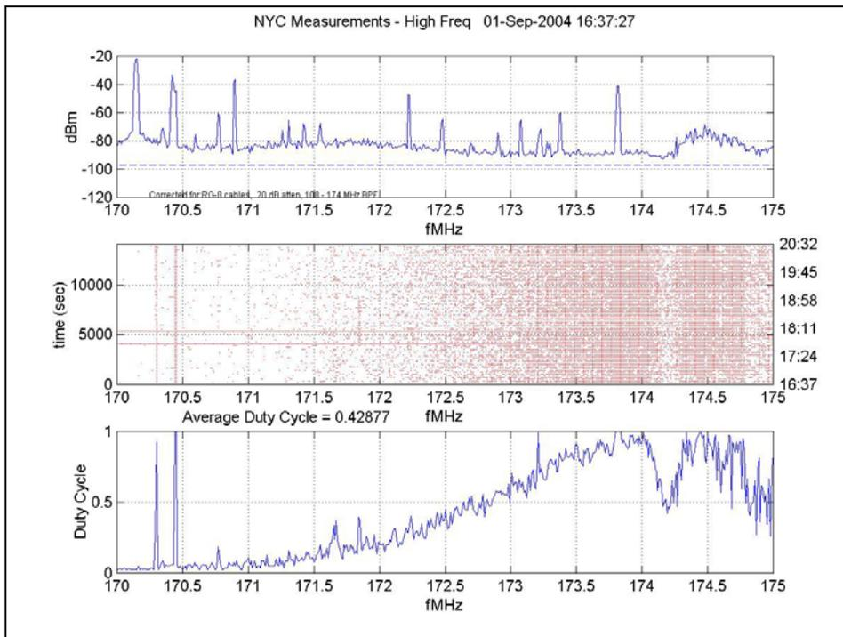
Figure 89: Small Frequency Resolution, 170 MHz – 175 MHz
