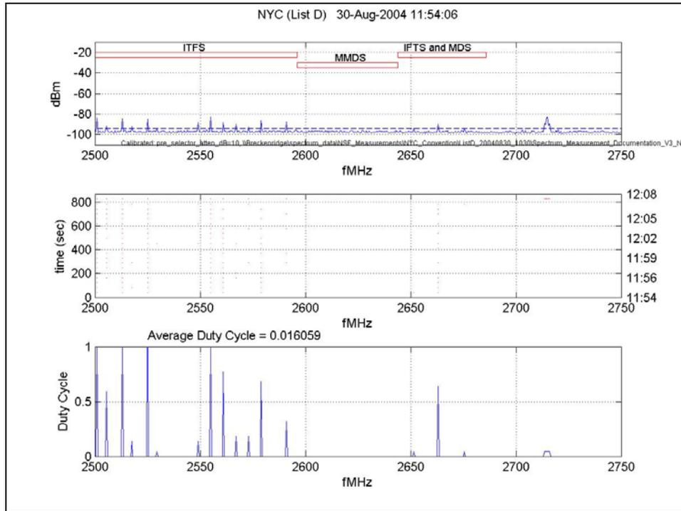
Figure 166: Large Signal Data, 2500 MHz – 2750MHz
