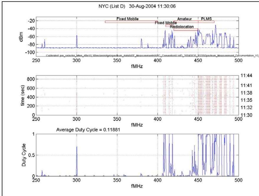
**Figure 157: Large Signal Data, 250 MHz – 500 MHz**
