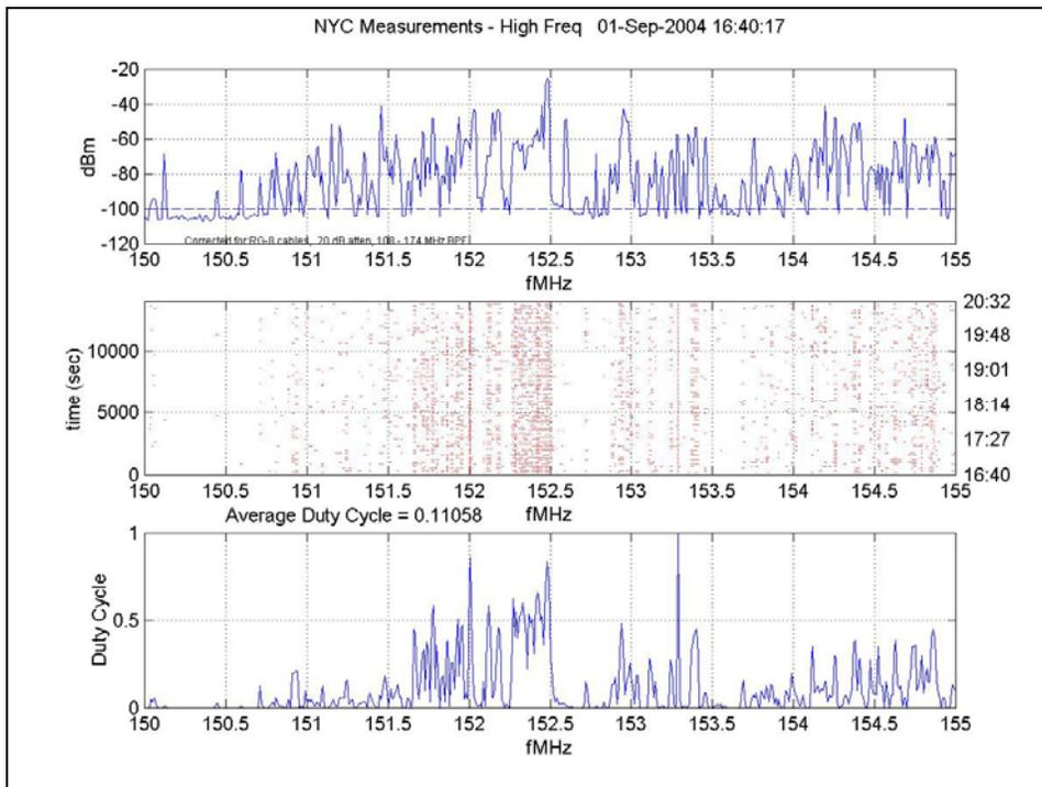
Figure 85: Small Frequency Resolution, 150 MHz – 155 MHz
