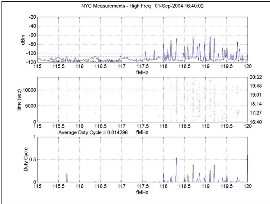
Figure 78: Small Frequency Resolution, 115 MHz – 120 MHz
