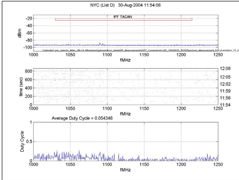
Figure 160: Large Signal Data, 1000 MHz – 1250 MHz
