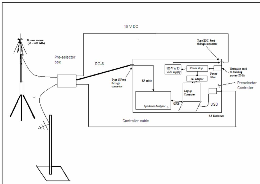
**Figure 1: Spectrum Measurement Equipment Configuration**
