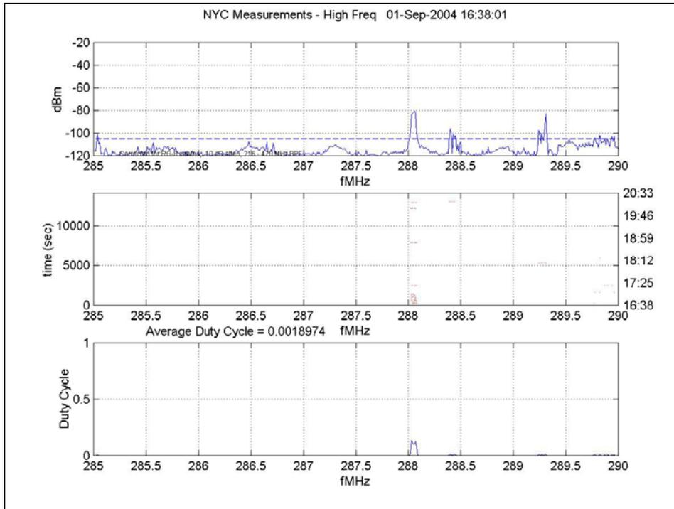
Figure 106: Small Frequency Resolution, 285 MHz – 290 MHz
