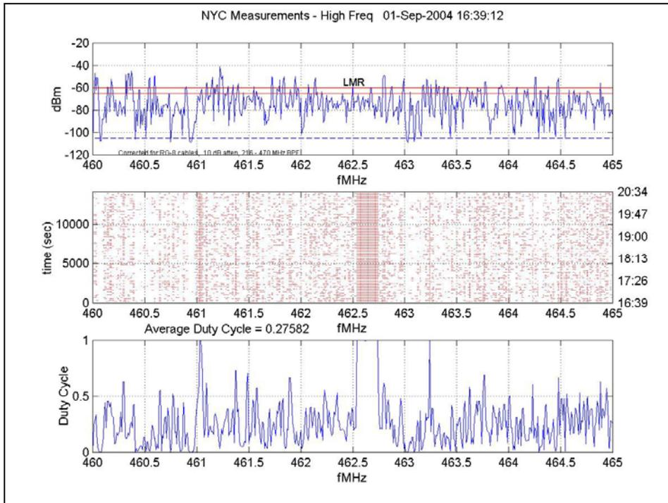
Figure 141: Small Frequency Resolution, 460 MHz – 465 MHz
