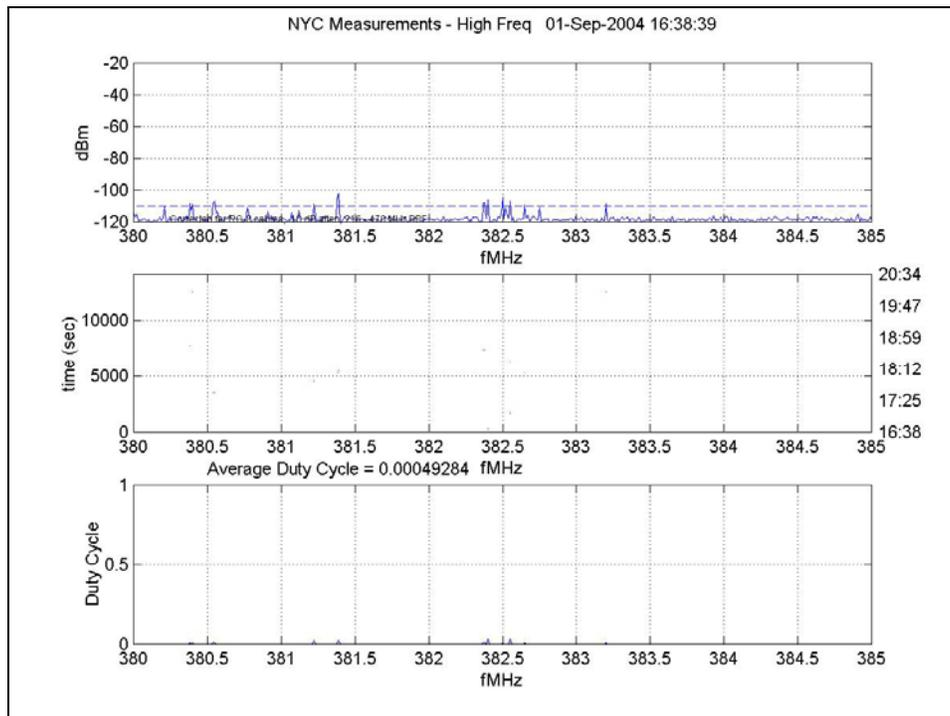
Figure 125: Small Frequency Resolution, 380 MHz – 385 MHz
