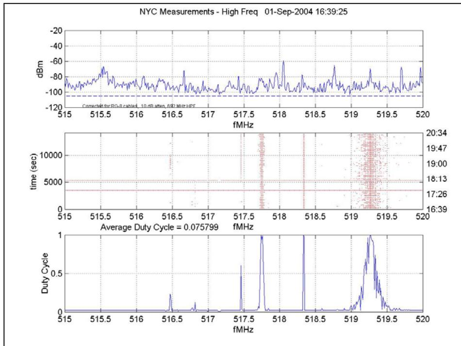
Figure 147: Small Frequency Resolution, 515 MHz – 520 MHz
