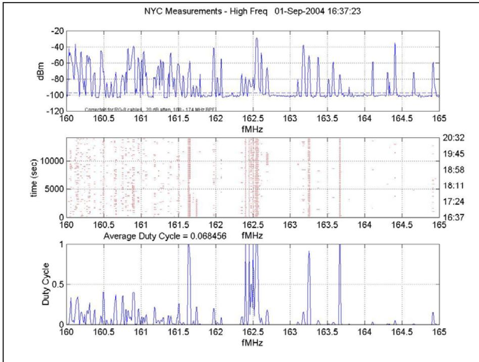
Figure 87: Small Frequency Resolution, 160 MHz – 165 MHz
