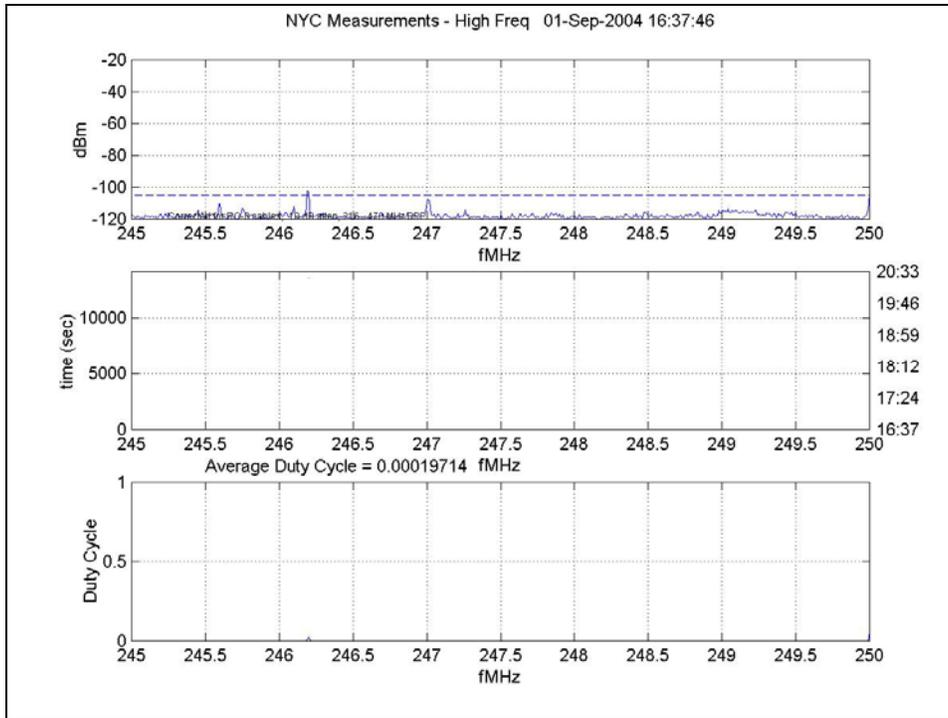
Figure 98: Small Frequency Resolution, 245 MHz – 250 MHz
