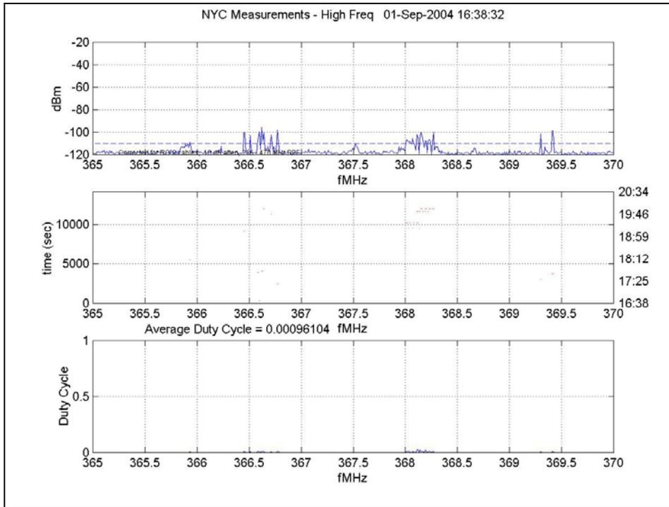
Figure 122: Small Frequency Resolution, 365 MHz – 370 MHz
