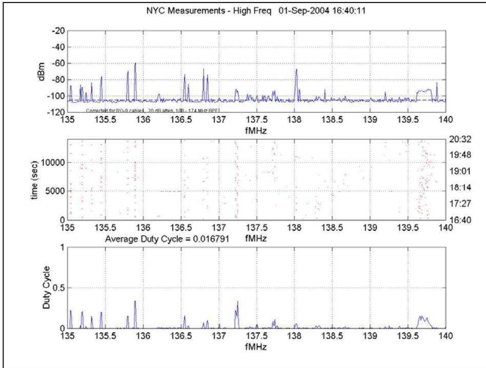
Figure 82: Small Frequency Resolution, 135 MHz – 140 MHz
