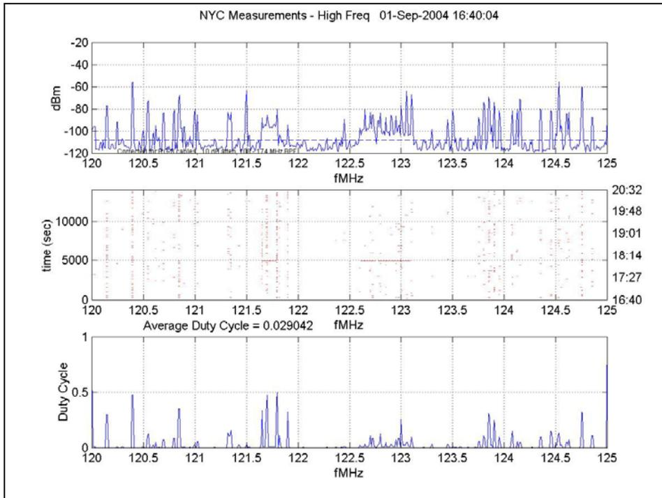
Figure 79: Small Frequency Resolution, 120 MHz – 125 MHz
