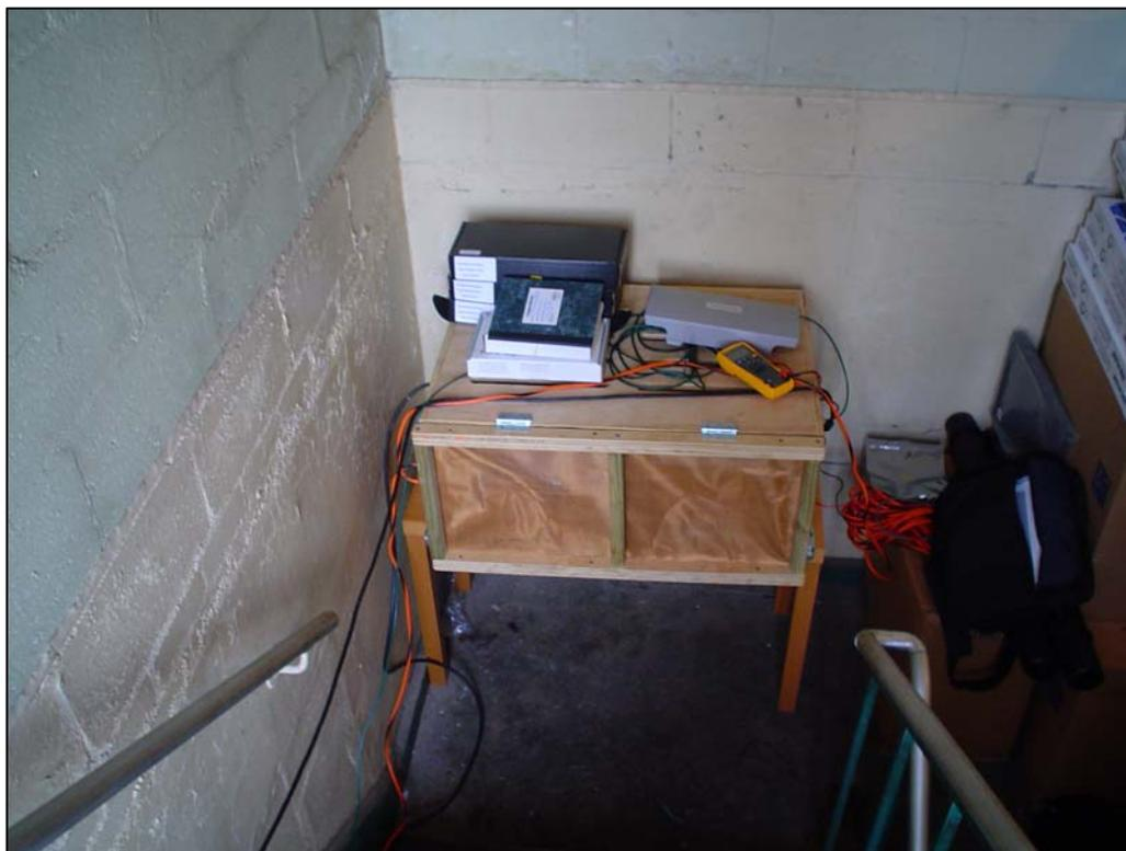
**Figure 3: RF Shielded Box Used to Reduce Emissions from Laptop and Spectrum Analyzer**
