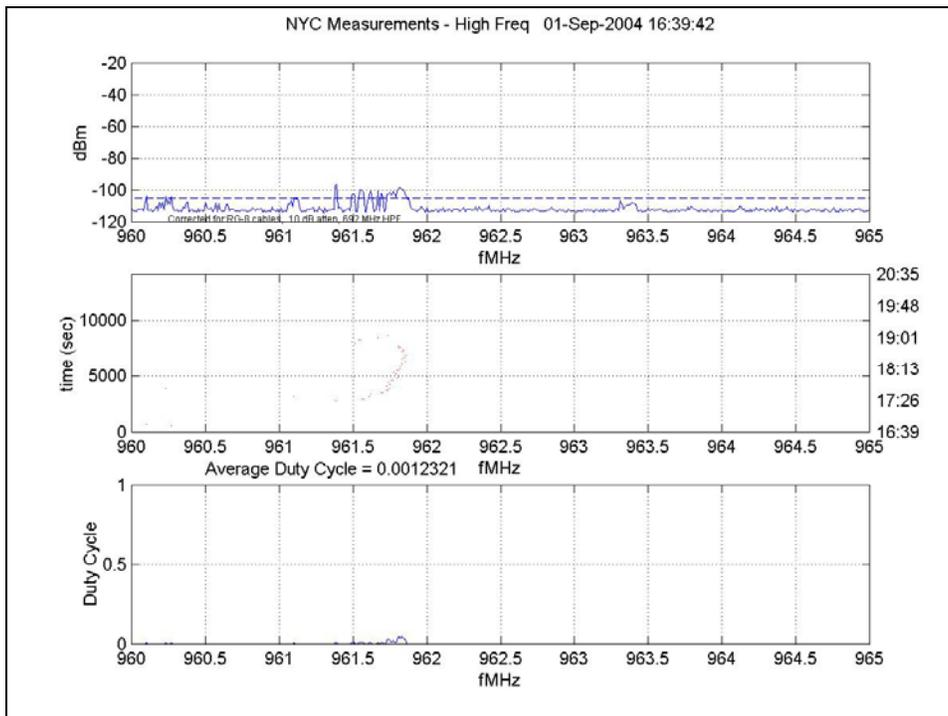
Figure 155: Small Frequency Resolution, 960 MHz – 965 MHz
