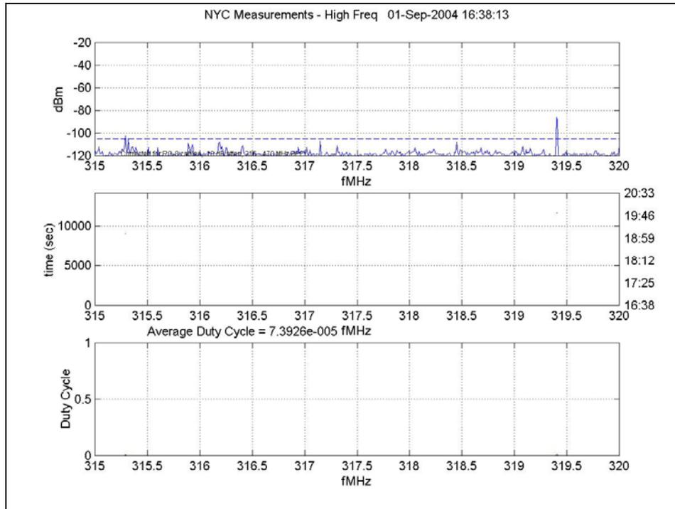
Figure 112: Small Frequency Resolution, 315 MHz – 320 MHz
