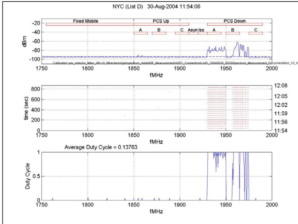
**Figure 163: Large Signal Data, 1750 MHz – 2000 MHz**
