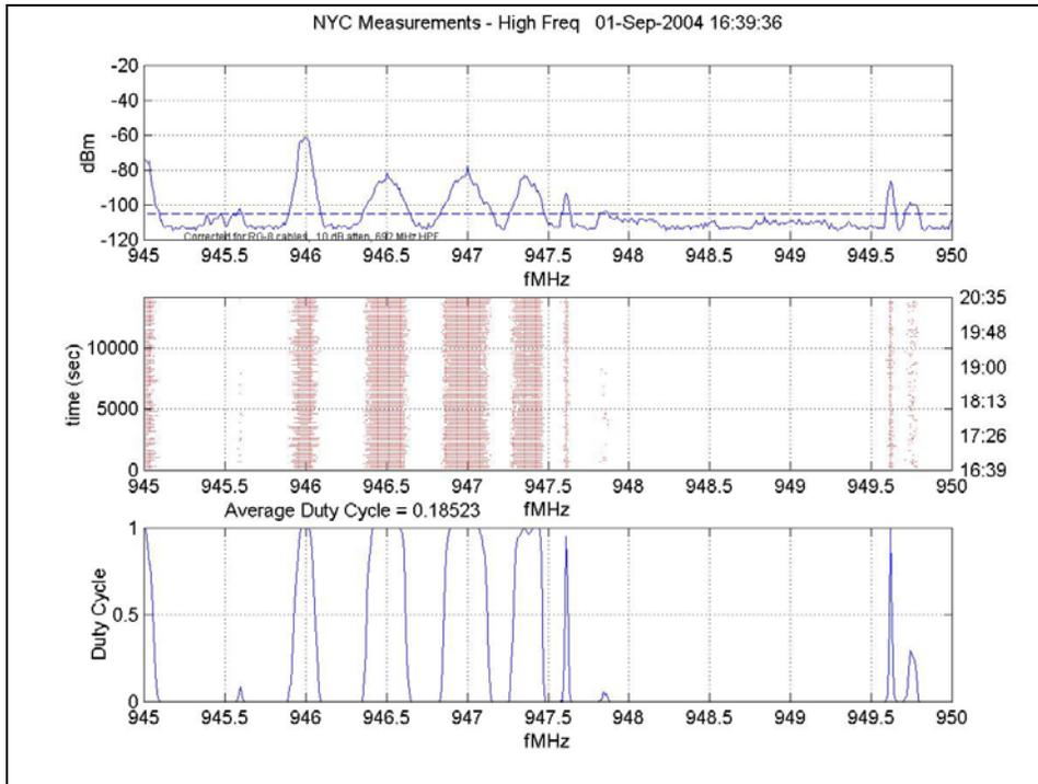
Figure 152: Small Frequency Resolution, 945 MHz – 950 MHz
