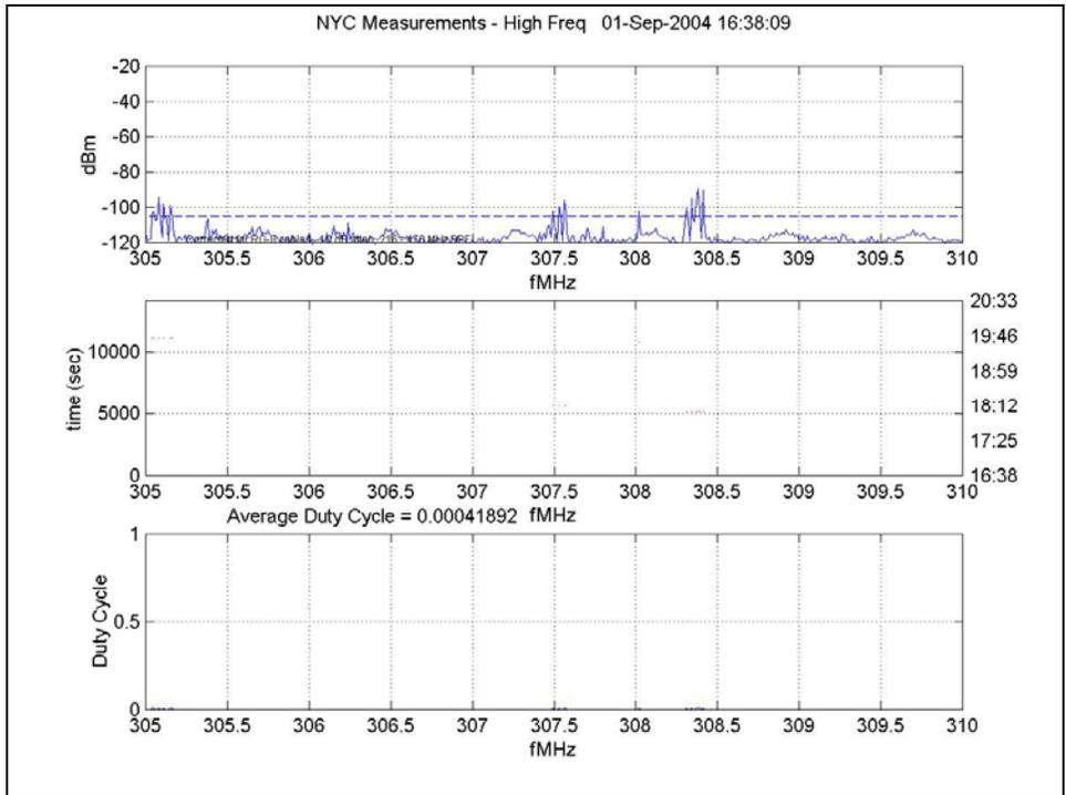
Figure 110: Small Frequency Resolution, 305 MHz – 310 MHz
