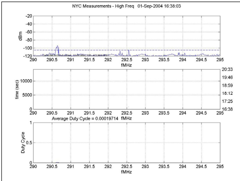
Figure 107: Small Frequency Resolution, 290 MHz – 295 MHz
