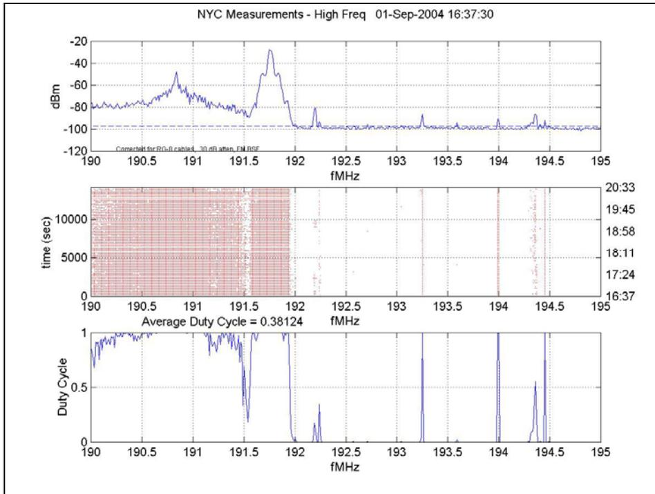
Figure 90: Small Frequency Resolution, 190 MHz – 195 MHz
