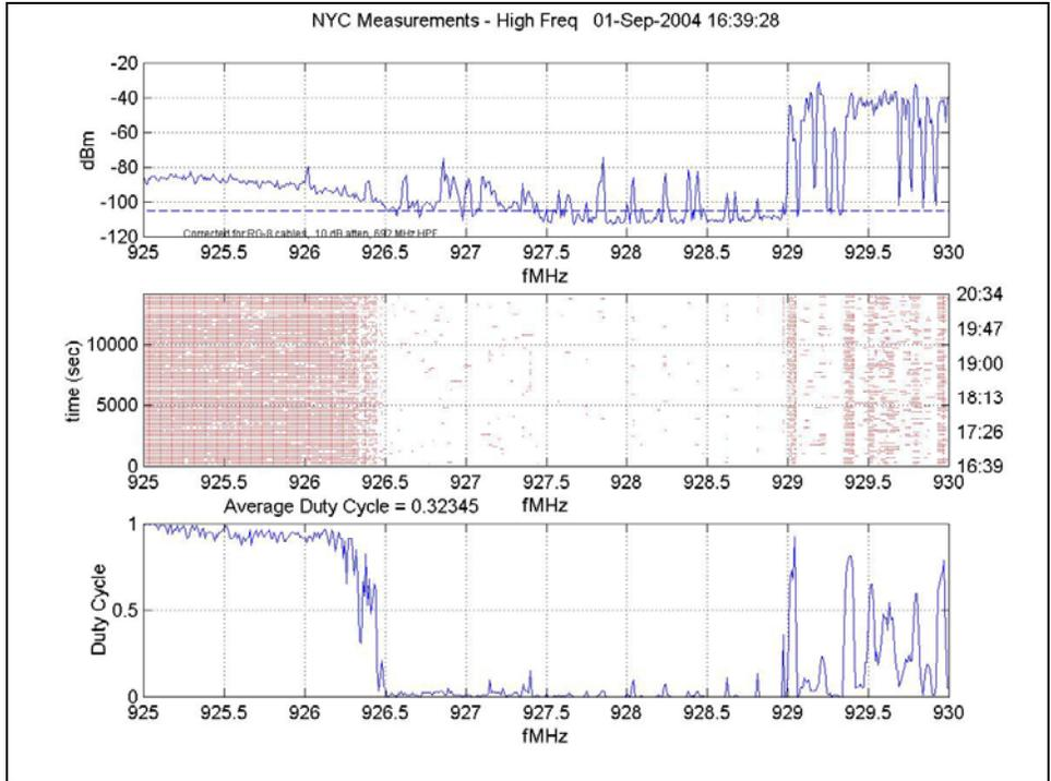
**Figure 148: Small Frequency Resolution, 925 MHz – 930 MHz**
