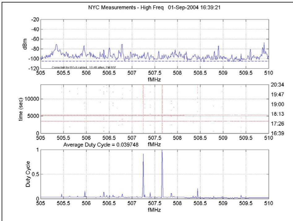
Figure 145: Small Frequency Resolution, 505 MHz – 510 MHz
