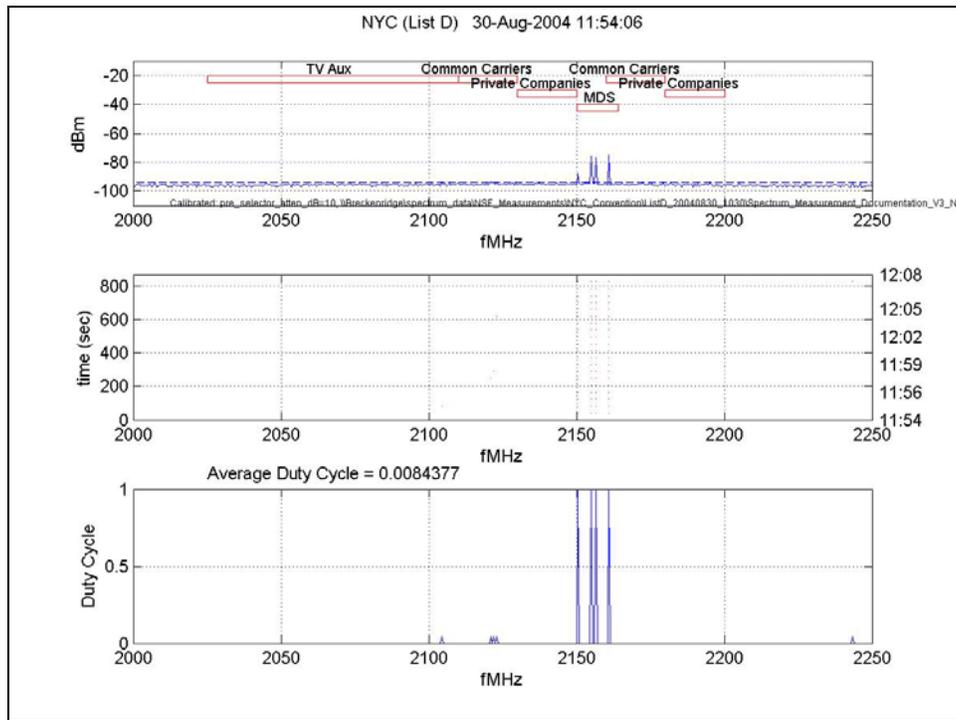
**Figure 164: Large Signal Data, 2000 MHz – 2250 MHz**
