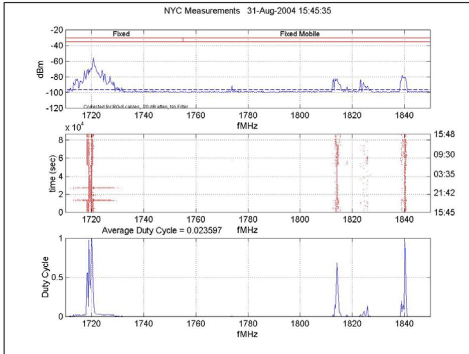
**Figure 50: August 31 to September 1, 1710 MHz – 1850 MHz**
