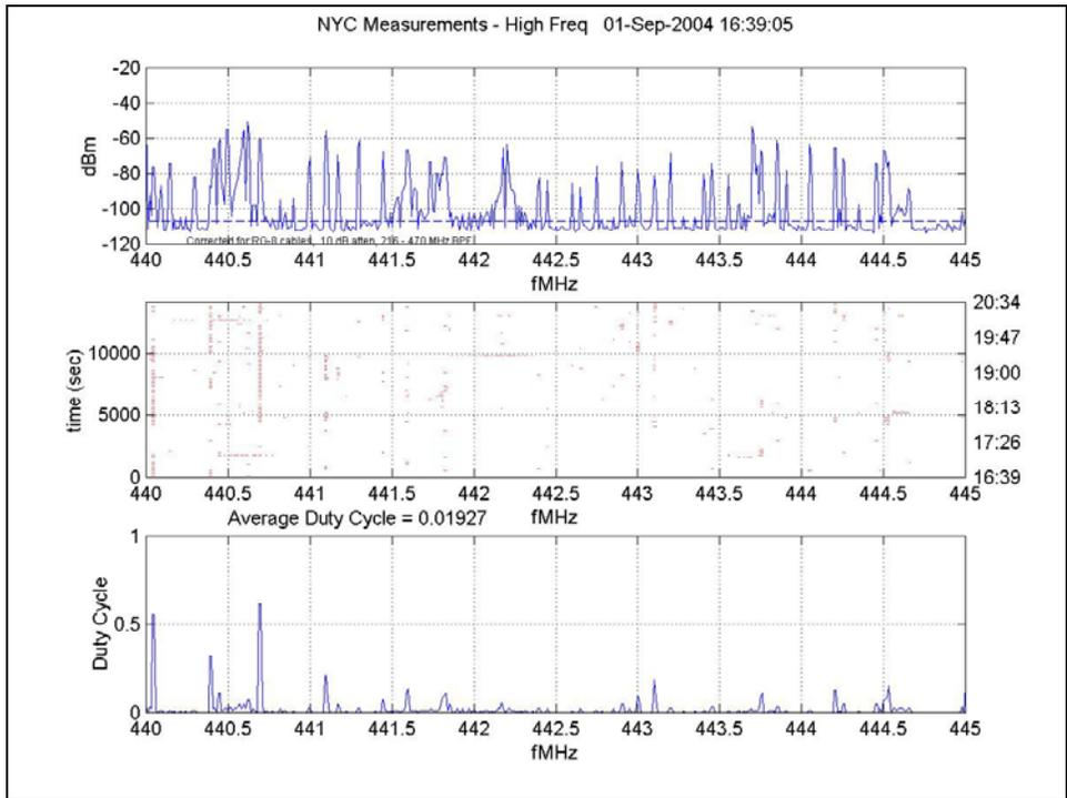
Figure 137: Small Frequency Resolution, 440 MHz – 445 MHz
