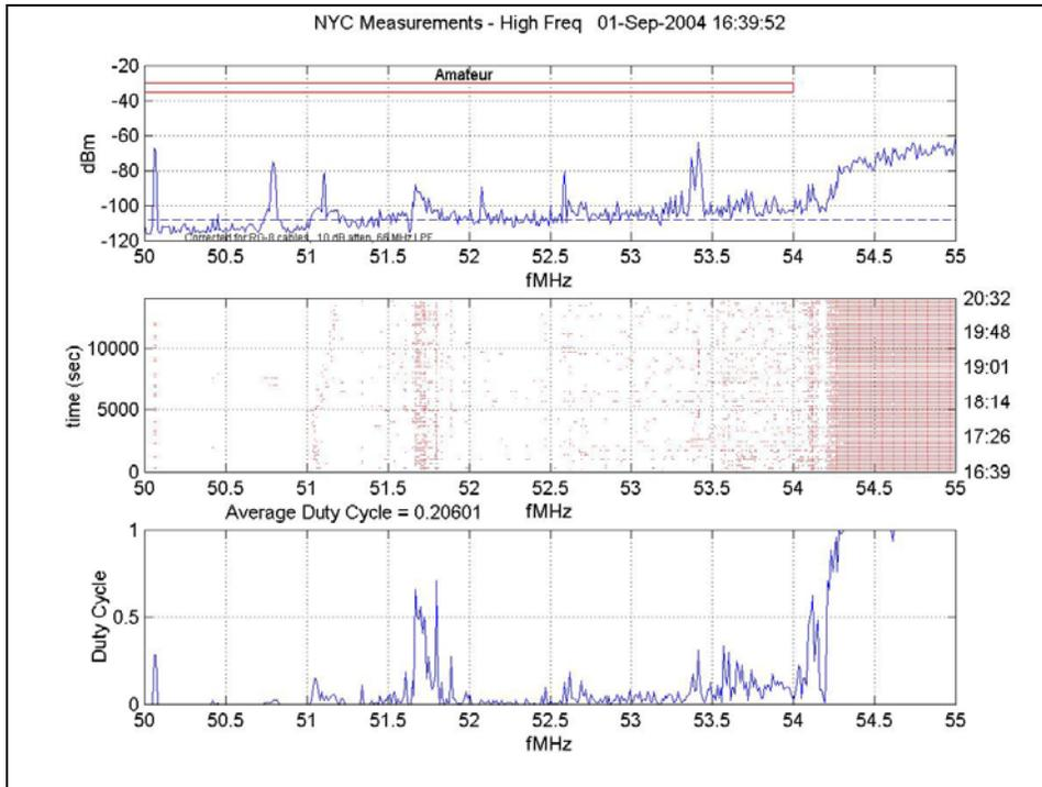
Figure 74: Small Frequency Resolution, 50 MHz – 55 MHz
