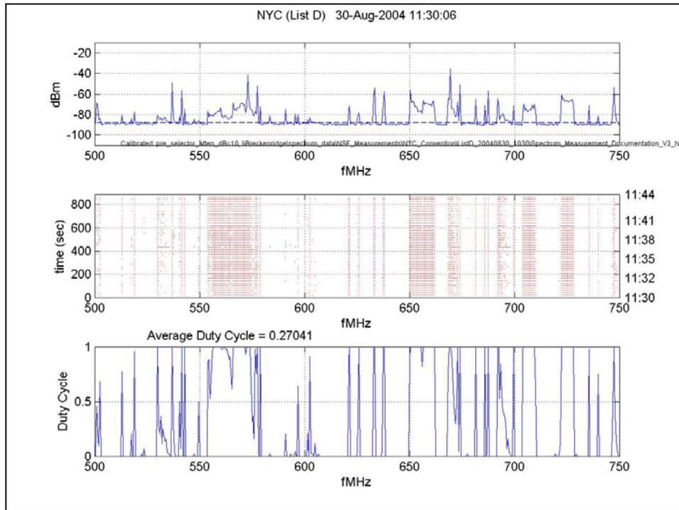
**Figure 158: Large Signal Data, 500 MHz – 750 MHz**
